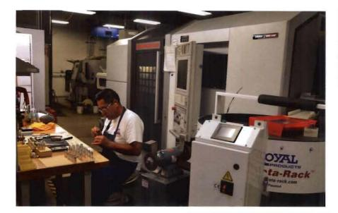
Donson Machine's operators and quality inspectors perform in-process inspection and audits to ensure consistent, high part quality. The shop commonly uses statistical process control (SPC) to ensure quality for both prototyping work and production runs.
