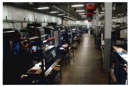
The shop has 60 machines, including VMCs, HMCs, and specialty and prototype milling machines. Some of its machining centers offer fourth- and fifth-axis capabilities, spindle speeds as high as 14,000 rpm and high-pressure coolant. Donson Machine uses pallet changers, tombstones and other quick-change fixtures and tooling to reduce setup and production cycle time and improve machine/operator utilization.
